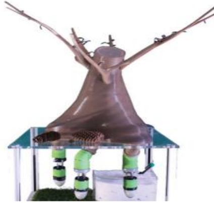
Fig. 5. The plantoid: a bioinspired robot developed at the Italian Institute of Technology, Pisa, Italy, by The Plantoid Project led by Barbara Mazzolai. © Bioinspired Soft Robotics Lab, Italian Institute of Technology, Pisa, Italy.
