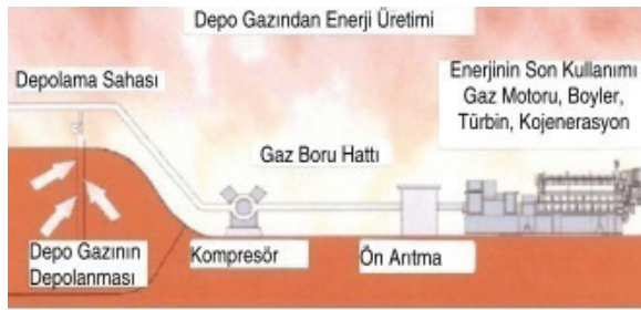
Figure 1. Energy generation system from landfill gas [16]
