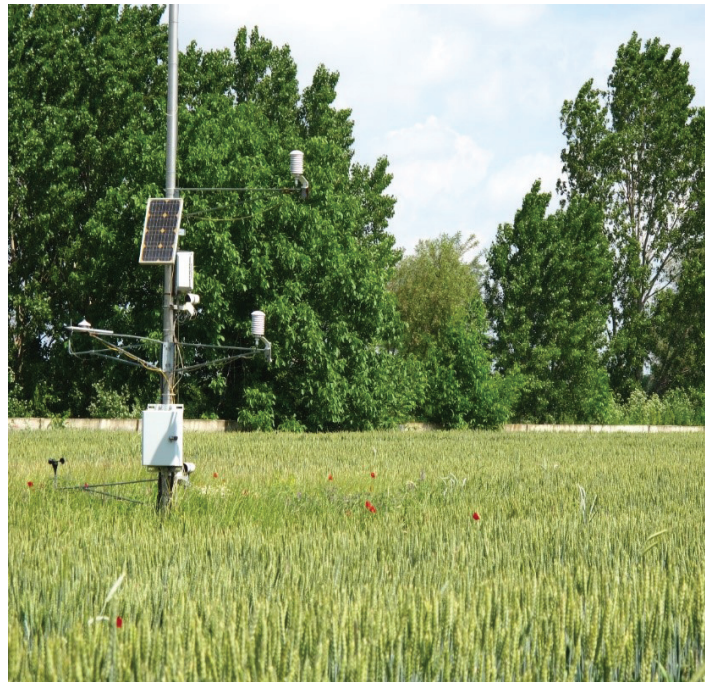
Figure 2. BREB measurement system.
