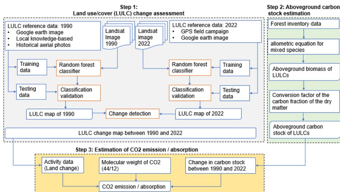
**Fig.2.** Process for estimating CO<sub>2</sub> emission from LULC change in the municipality of Ouagadougou
